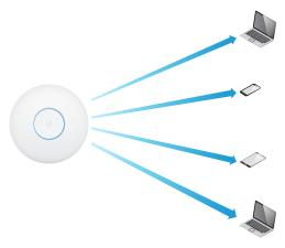
MU-MIMO with 1x1 clients: The UniFi AC HD AP communicates with four 1x1 clients at a time.
