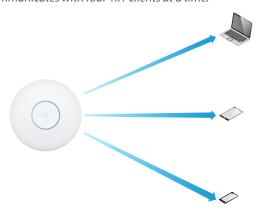
MU-MIMO with 2x2 and 1x1 clients: The UniFi AC HD AP communicates with one 2x2 client and two 1x1 clients at a time.
